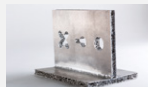
Further processing options: drilling, welding, milling
