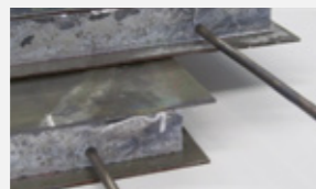
Steel-aluminum foam sandwiches with steel pipe
