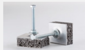
SAS manufacturing technology: directly foamed-bolts and nuts
