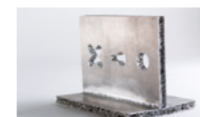
Further processing: Drilling, welding, milling
