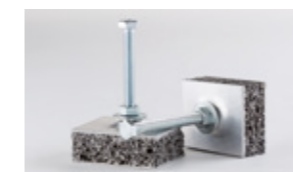
SAS production technology: Direct inclusion of bolts and nuts
